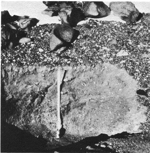
FIGURE 7 Soil of the trough of a poorly expressed, nonsorted polygon (Profile 36), Beacon Valley. The soil shows diffuse bands imparting differences in color. The massive structure and the weak coherence is responsible for maintaining a vertical face and for preventing the soil material to flow.
