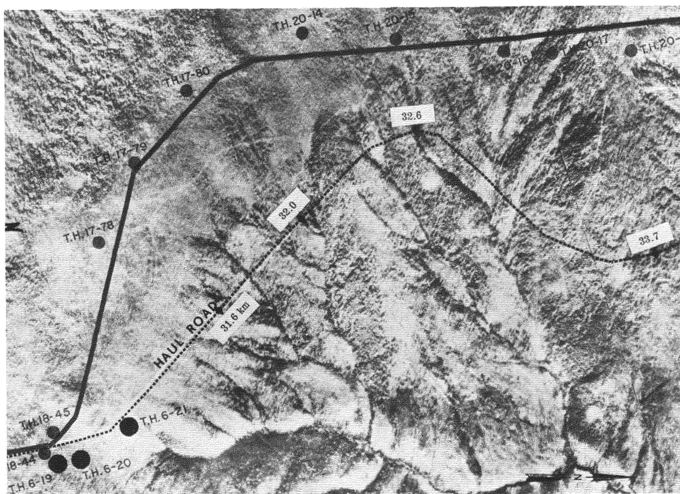
FIGURE 2 Locations of cuts in high-ice-content soils along roadway. 1 The solid line is the alignment of the proposed 1.22-m pipeline; soil test holes are indicated by the T.H. followed by numerals.
