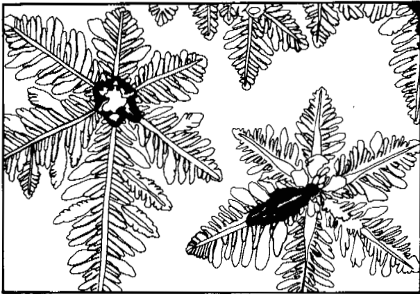
Fig. 2. Snowflake-shaped Tyndall figure in a large crystal of glacier ice subjected to strong radiation. (From Nakaya, 1956, Plate 9, No. 22. )
