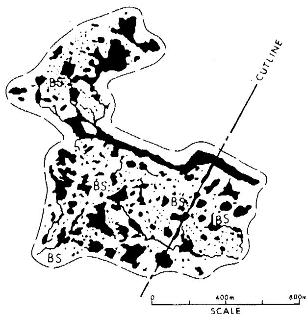
FIG. 2 Speckled bog terrain (BS) (peat plateau) showing areal extent of permafrost (white) and thawed collapse bogs (black).
