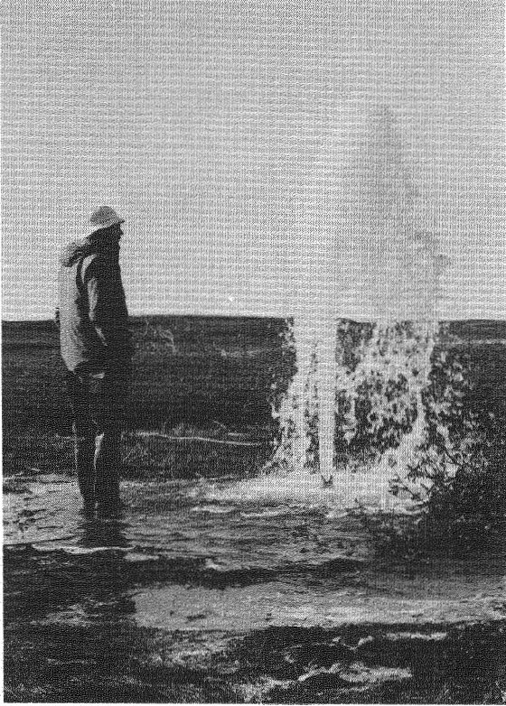
Figure 4. Drill hole flow in 1977 from pingo 14. The water came from a depth of 22 m and jetted up 2.6 m high from a 7.5 cm diameter hole. The clear mineralized water had an orifice temperature of about -0.1^{\circ}\text{C} .
