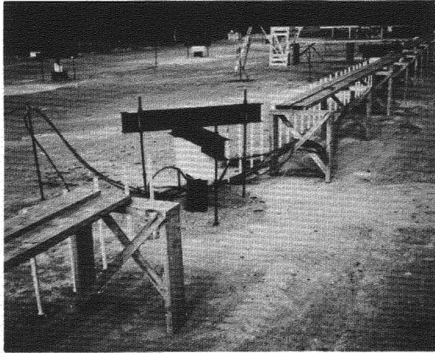
FIGURE 3 Test site, showing reaction frames with insulated force gauges, catwalk, instrument trailers, Stevenson screen, and thermocouple cables.
