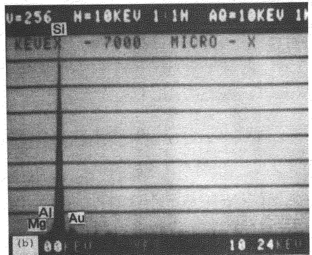
Fig. 4. SEM image (a) and EDX analysis (b) of sand from Hyannis, Massachusetts.
