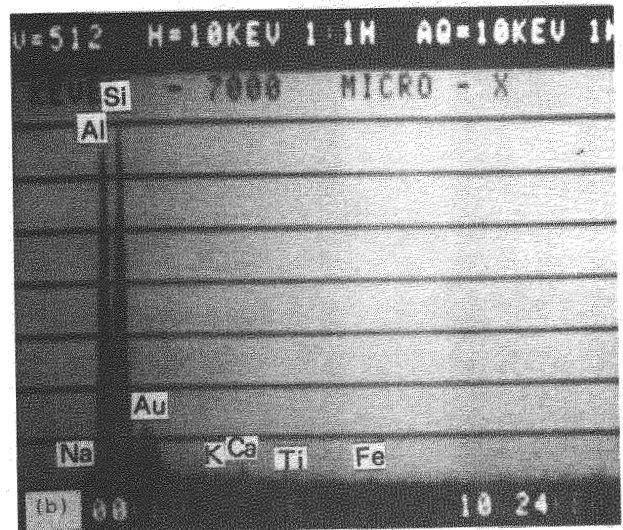
Fig. 3. SEM image (a) and EDX analysis (b) of dickite from San Juanito, Mexico.
