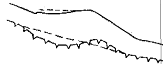
Figure 5. Thaw settlement in highway slope section
