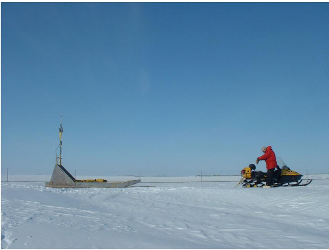
Figure 3. DGPS equipment mounted on a sled behind a snow machine (April 2005).
