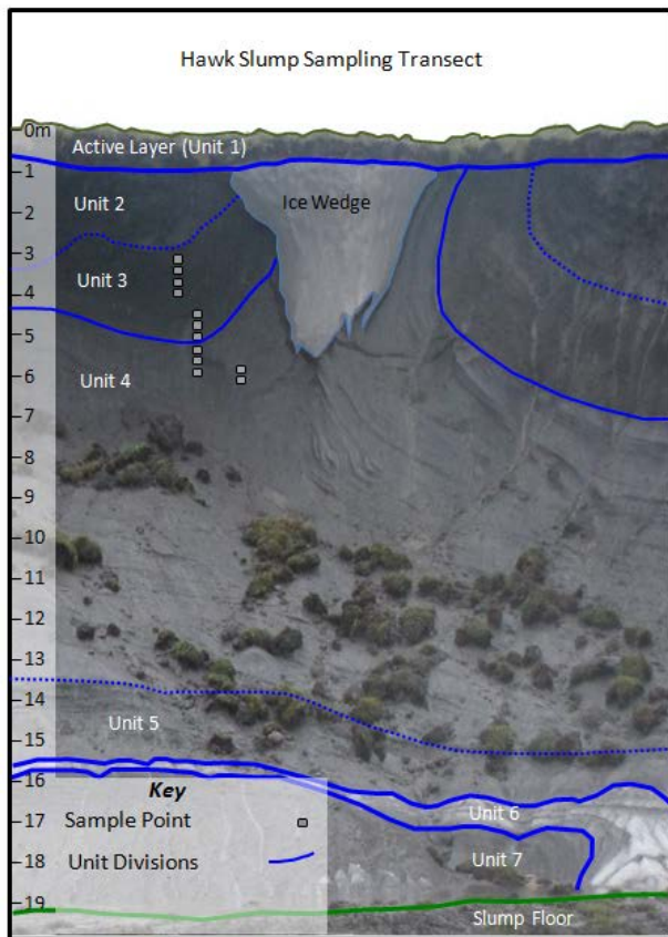
Figure 3. In order to correspond to CCR's depth of investigation, only sampling results from the upper 8 m of the subsurface are discussed in this paper (unit 3 and part of unit 4). Unit 3 is classified as ice-poor silty clay (2.5–4.0 m) and massive ice is represented in unit 4 (4.0–13.5 m).
