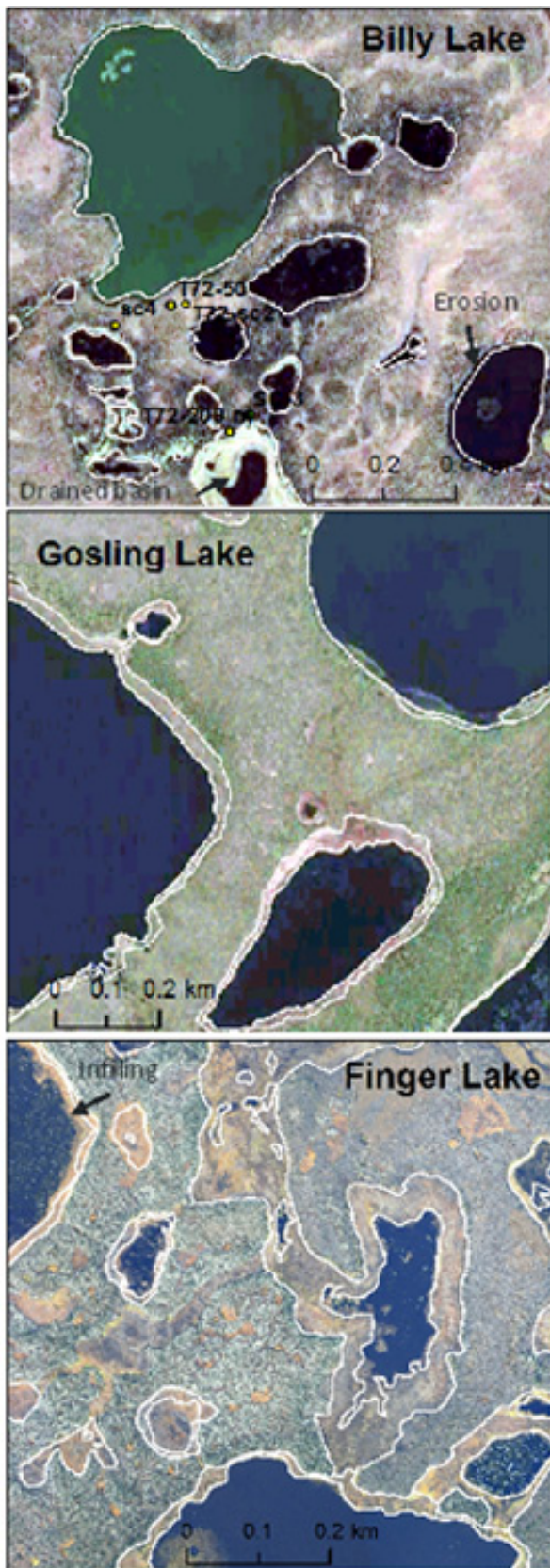
Figure 5. Lake and shore fen boundaries (white) from circa 1950 overlaid on recent imagery showing changes in thermokarst.
