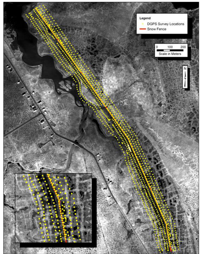
Figure 4. Location of 1264 DGPS measurement points collected along five transects in April 2005. Middle transect as bold line.
