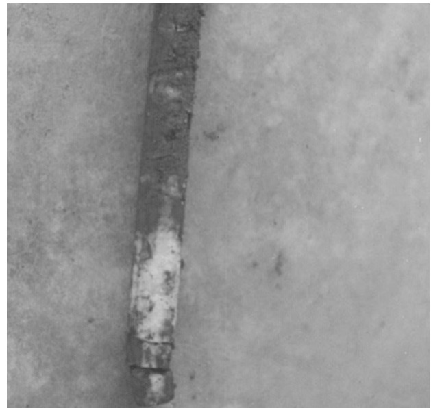
Figure 3b. Recovered frozen core sample containing an ice seam taken from Test Hole TH-1 (see Fig. 2).
