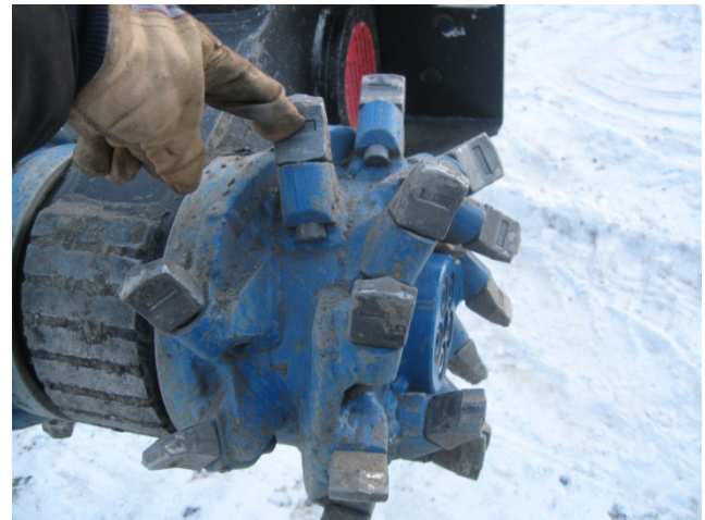
Figure 4. One drum of the EC-25 installed with chisel type picks
