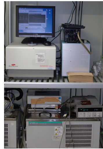
Figure 2. P-NMR System (MARAN Ultra with temperature bath).
