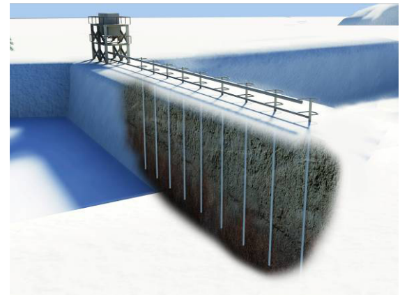
Figure 10. Liendokit River dam with deep foundation and a seasonally cooling device of a collector type.
