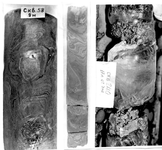
Figure 3. Ground ice in the dislocated subsea sediments of the Barents-Kara Shelf (Melnikov & Spesivtsev 1995, Bondarev et al. 2001).
